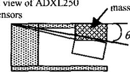
Fig. 2(c) Mass on a Cantilever
