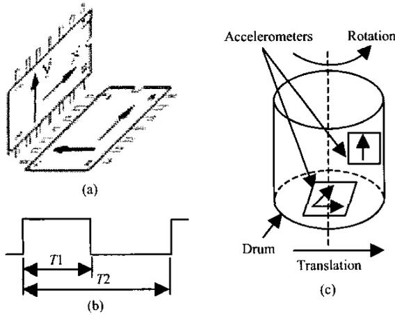
Fig. 3 Accelerometers Mounted on Drum
